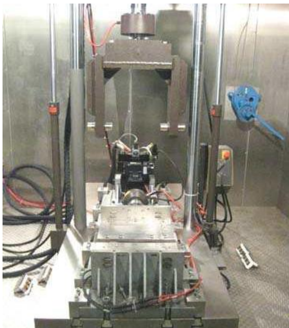
Figure 17. Movement testing at -40° to +60°C
