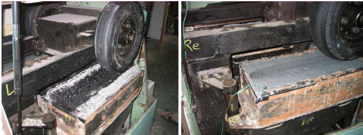
Figure 16. Comparison of flexible plug joint materials after rutting test acc. to EN 12697-22 at 60°C (Left: Common asphalt plug material after 100 cycles. Right: Polyflex® Advanced after 30,000 cycles)
