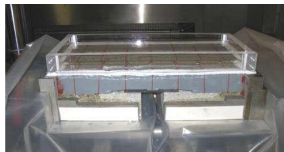
Figure 18. Verification of watertightness (at maximum opening position of joint) following movement capacity test
