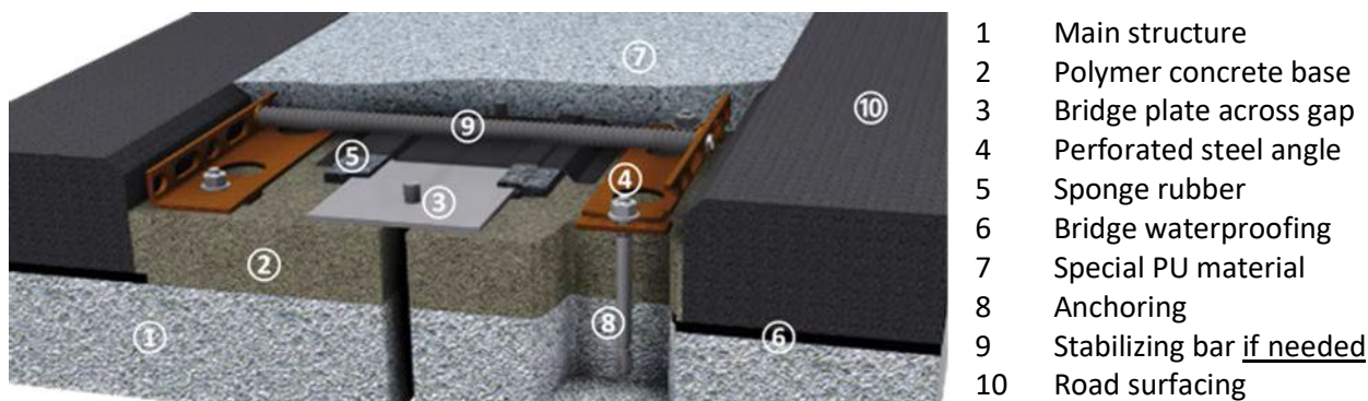
Figure 2. Illustration showing the main elements of a typical Polyflex®Advanced expansion joint
