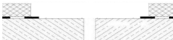
Figure 6. Arrangement of ends of waterproofing membrane in recess
