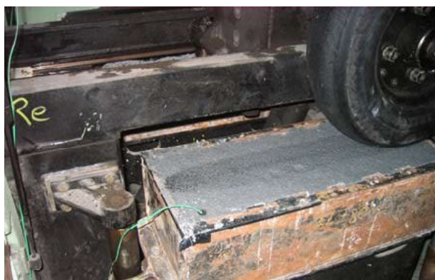
Figure 11. Comparison of flexible plug materials after rutting test per EN 12697-22 at 60°C. Above: Common asphalt plug after 100 cycles. Below: Polyflex® Advanced after 30,000 cycles.
