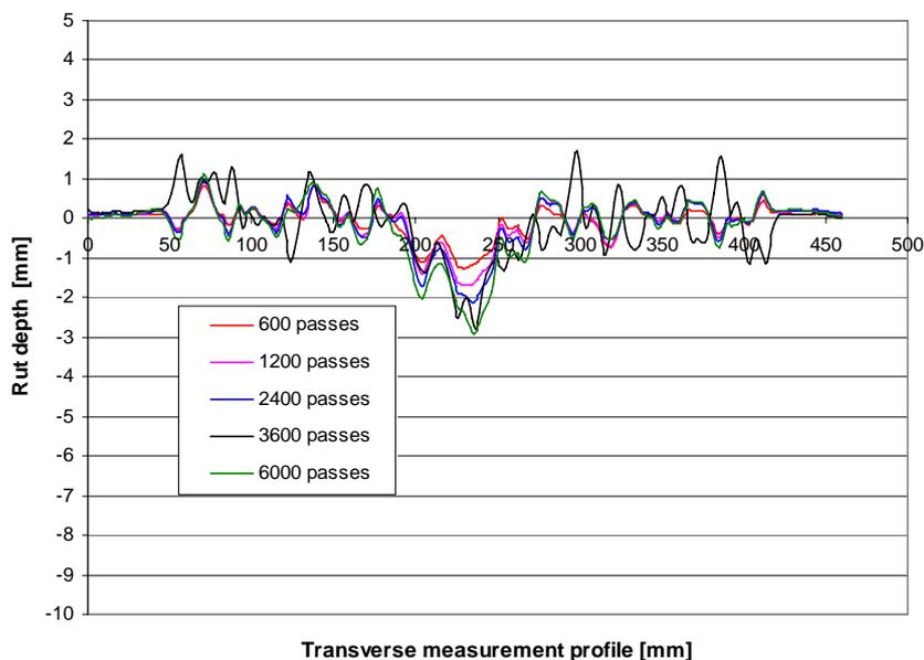
Figure 6.2.7: Diagram of rut depth measurements of the APJ A58-2 on profile 1 (in the middle of the APJ)
