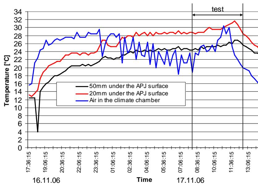
Figure 6.2.4: Diagram of the temperature measurement during the test of the APJ A58-1
