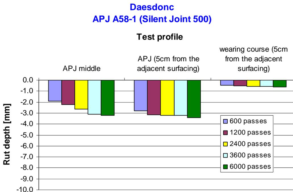
Figure 4.2.1: Result of rut depth measurements of the APJ A58-1 (wearing course: ZOAB and Densith)
