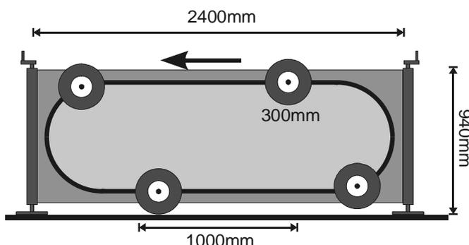
Figure 3.1.1: Schematic of MMLS3 testing rig
