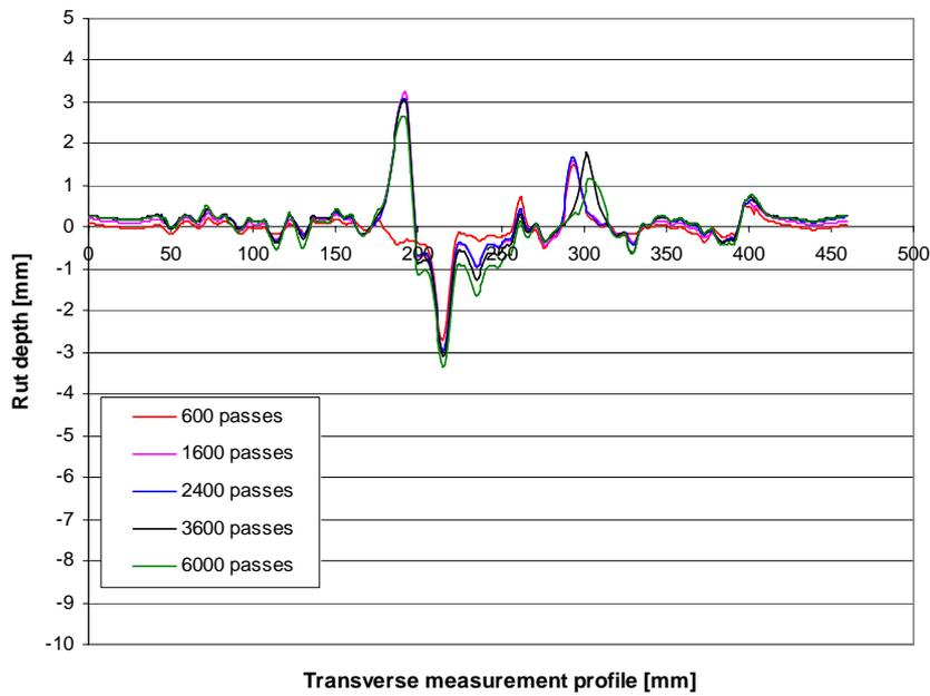
Figure 6.1.3: Diagram of rut depth measurements of the APJ A18-1 on profile 1 (in the middle of the APJ)
