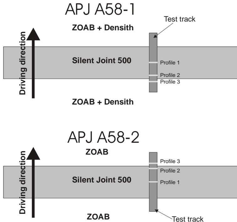
Figure 3.3.1: Location of the profile measurements of the APJ A58-1 and A58-2 on the bridge A58 Daesdonc
