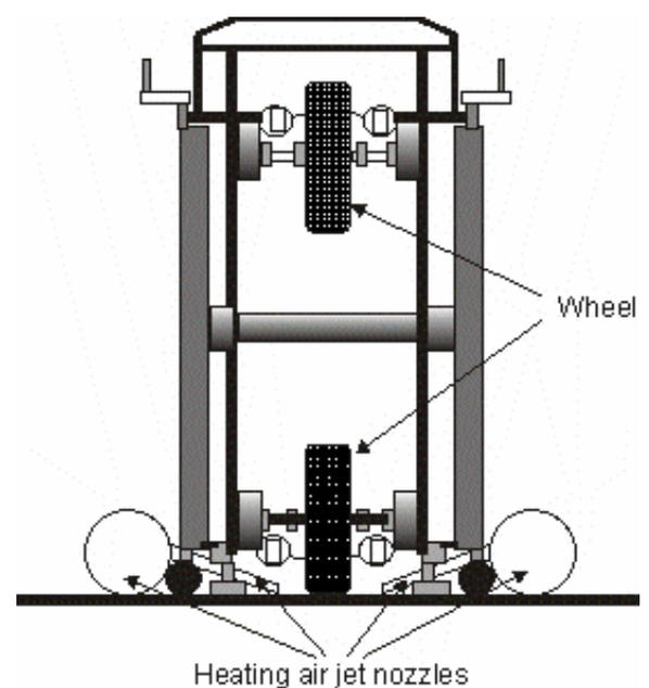
Figure 3.1.2: Position of the heating air jets
