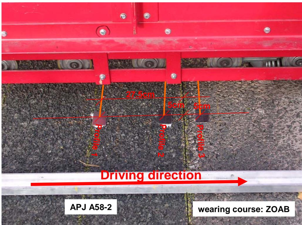
Figure 6.3.8: Test profiles of the APJ A58-2
