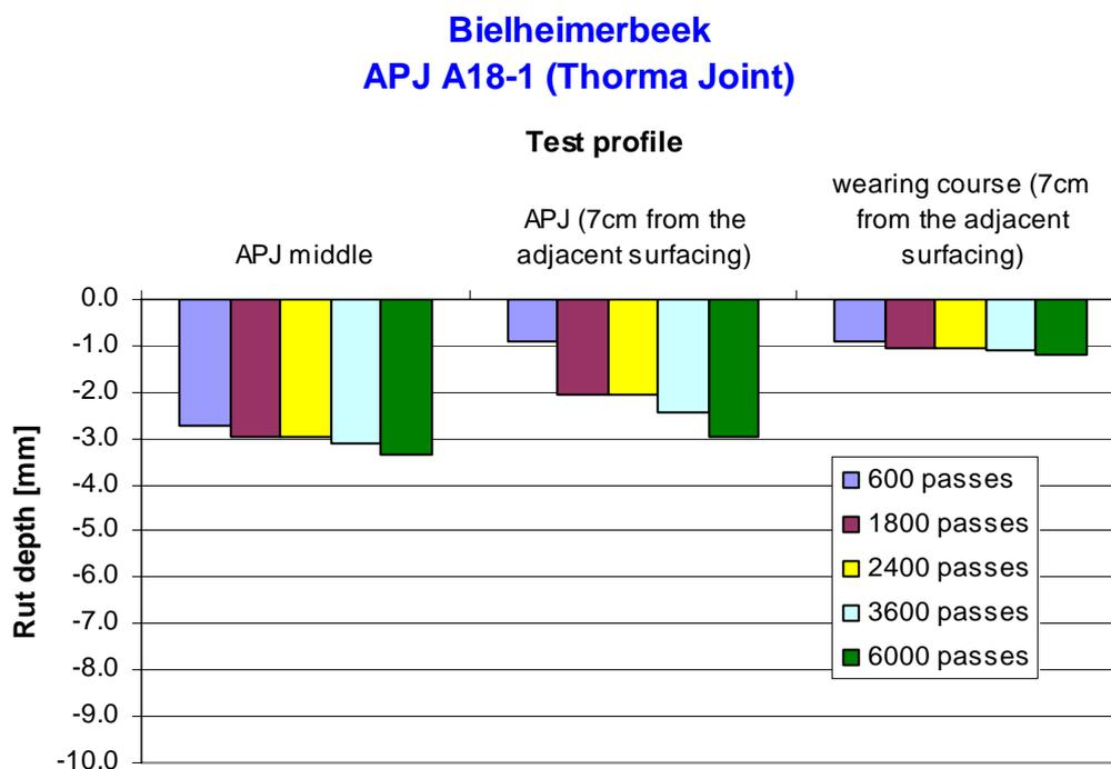
Figure 4.1.1: Result of rut depth measurements of the APJ A18-1 (wearing course: ZOAB)
