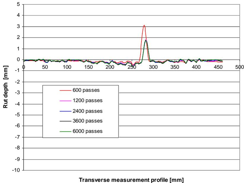
Figure 6.2.1: Diagram of rut depth measurements of the APJ A58-1 on profile 3 (on wearing course, about 5cm from the adjacent pavement surfacing)
