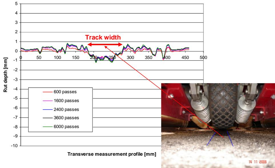
Figure 6.1.1: Diagram of rut depth measurements of the APJ A18-1 on profile 3 (on wearing course, about 7cm from the adjacent pavement surfacing)
