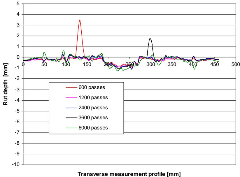
Figure 6.2.5: Diagram of rut depth measurements of the APJ A58-2 on profile 3 (on wearing course, about 5cm from the adjacent pavement surfacing)
