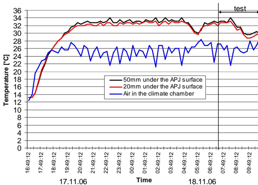
Figure 6.2.8: Diagram of the temperature measurement during the test of the APJ A58-2
