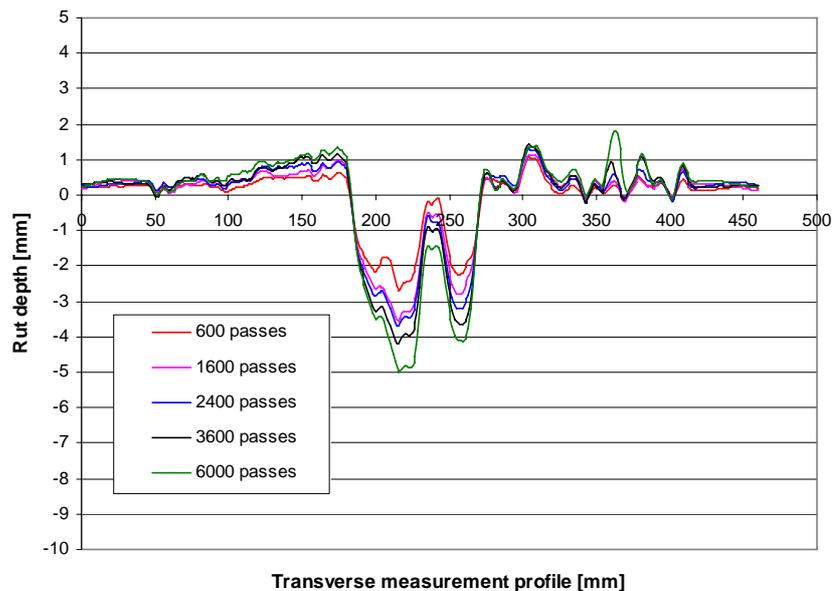
Figure 6.1.6 Diagram of rut depth measurements of the APJ A18-2 on profile 2 (on the APJ, about 7cm from the adjacent pavement surfacing)
