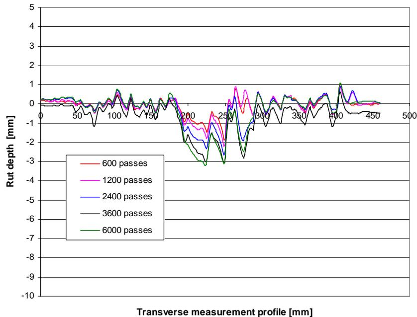
Figure 6.2.3: Diagram of rut depth measurements of the APJ A58-1 on profile 1 (in the middle of the APJ)
