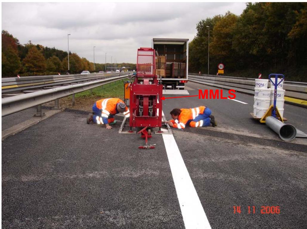
Figure 6.3.4: Device installation for testing the APJ A18-2
