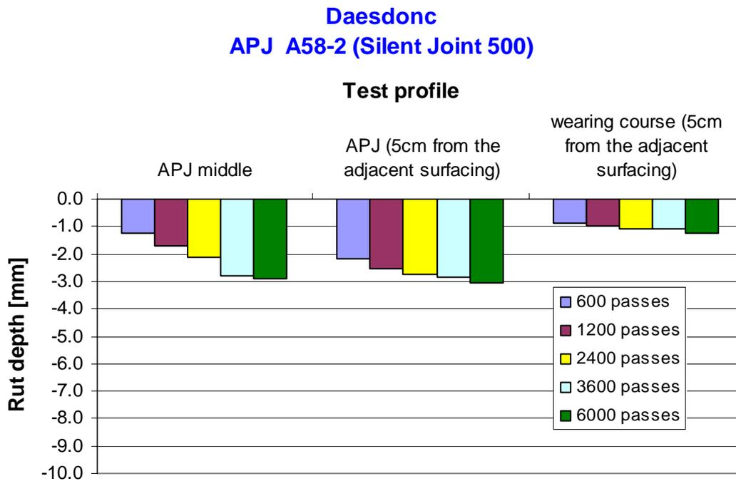
Figure 4.2.2: Result of rut depth measurements of the APJ A58-2 (wearing course: ZOAB)
