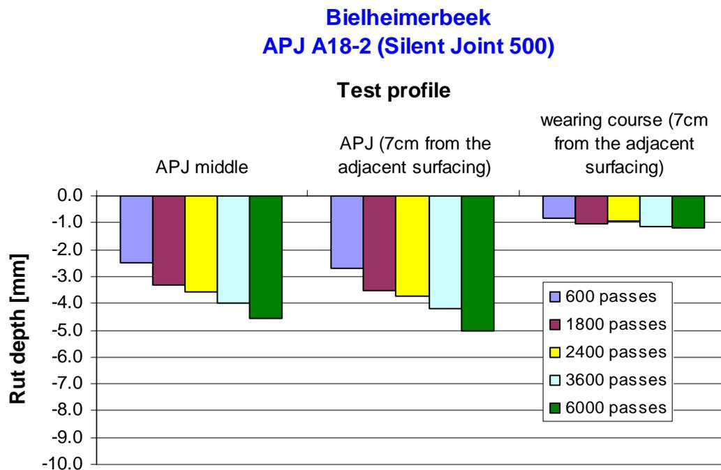
Figure 4.1.2: Result of rut depth measurements of the APJ A18-2 (wearing course: ZOAB)
