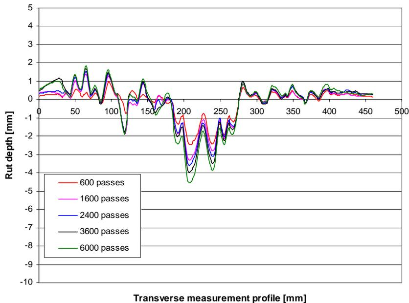
Figure 6.1.7: Diagram of rut depth measurements of the APJ A18-2 on profile 1 (in the middle of the APJ)
