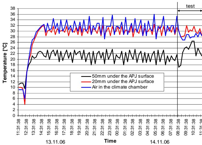
Figure 6.1.4: Diagram of the temperature measurement during the heating and the test of the APJ A18-2
