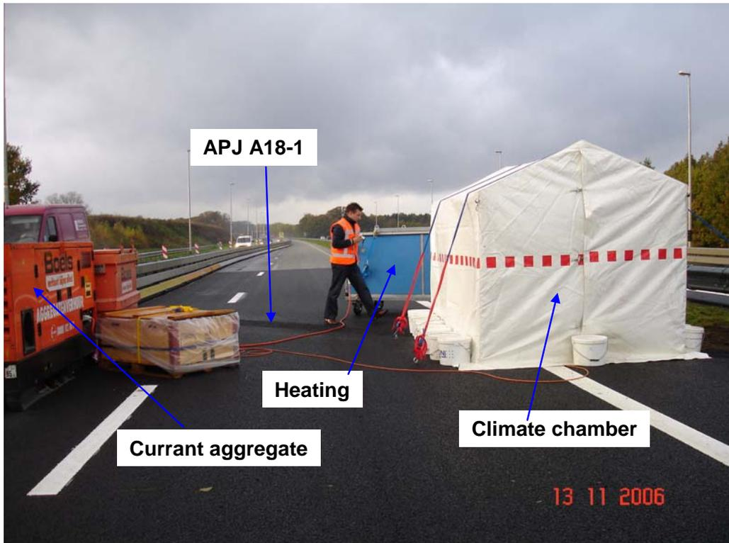
Figure 6.3.3: Test devices on the bridge Bielheimerbeek
