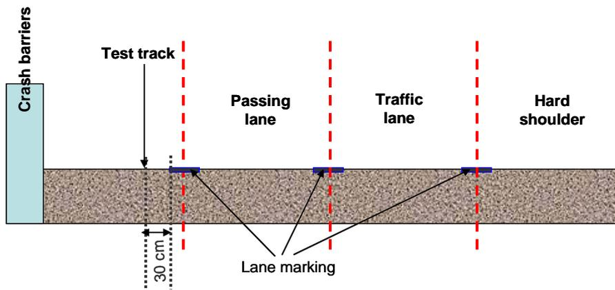
Figure 2.1.2: Test track on the bridge A18 Bielheimerbeek
