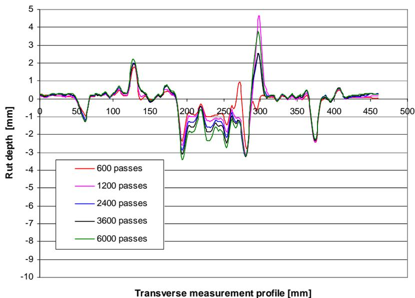
Figure 6.2.2 Diagram of rut depth measurements of the APJ A58-1 on profile 2 (on the APJ, about 5cm from the adjacent pavement surfacing)
