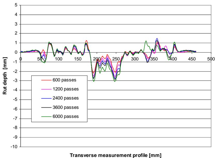
Figure 6.2.6 Diagram of rut depth measurements of the APJ A58-2 on profile 2 (on the APJ, about 5cm from the adjacent pavement surfacing)
