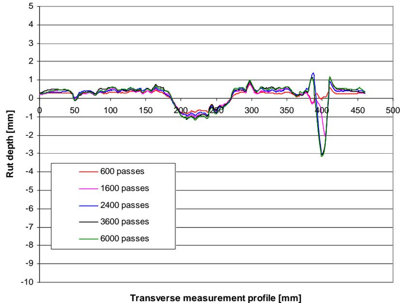
Figure 6.1.5: Diagram of rut depth measurements of the APJ A18-2 on profile 3 (on wearing course, about 7cm from the adjacent pavement surfacing)
