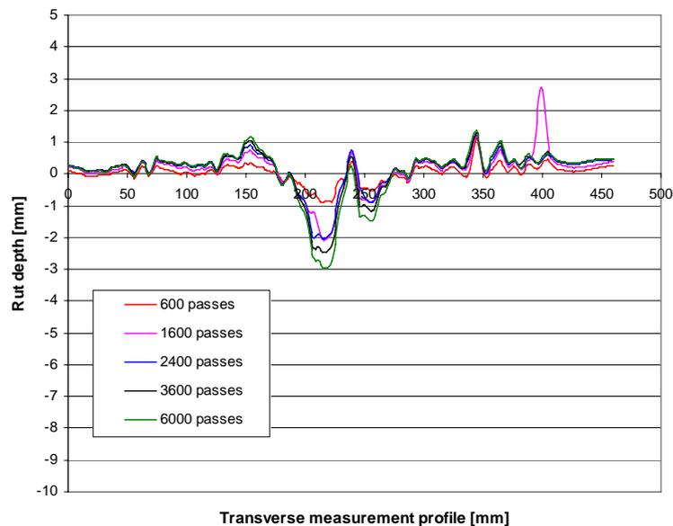
Figure 6.1.2: Diagram of rut depth measurements of the APJ A18-1 on profile 2 (on the APJ, about 7cm from the adjacent pavement surfacing)
