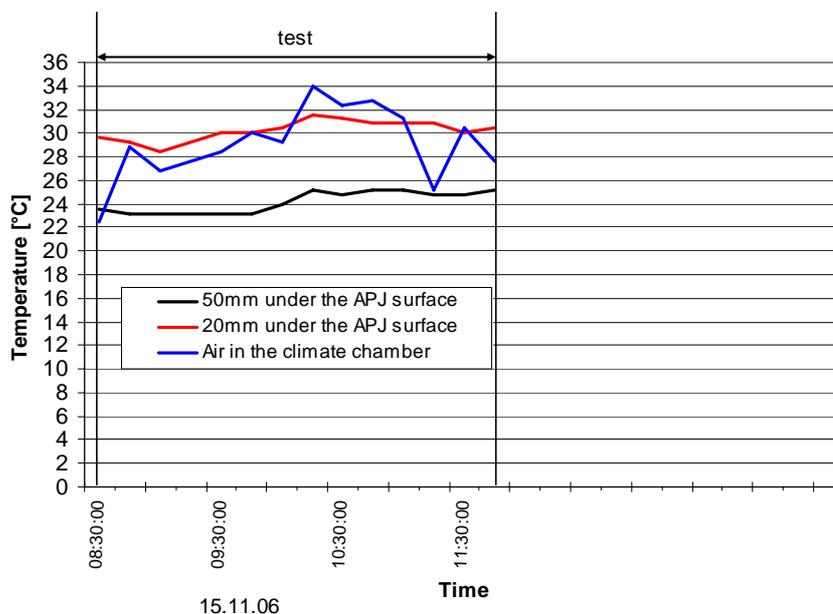
Figure 6.1.8: Diagram of the temperature measurement during the test of the APJ A18-2
