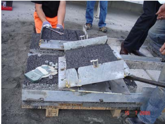
Figure 5.1.1: The prefab joint module was removed from its fixation's plate
