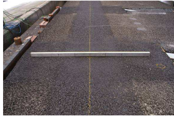
Rutting at N=60000. Left: +13 mm joint, right: -13mm joint.
