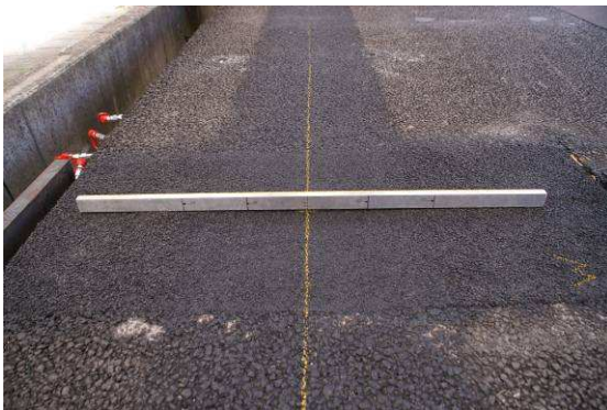
Rutting at N=40000. Left: +13 mm joint, right: -13mm joint.
