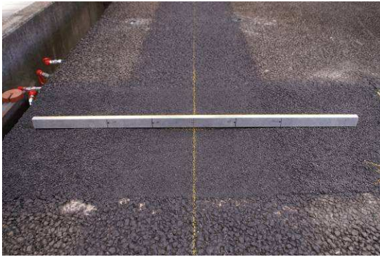
Rutting at N=60000. Left: +13 mm joint, right: -13mm joint.
