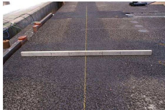
Rutting at N=10000. Left: +13 mm joint, right: -13mm joint.
