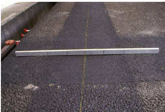
Rutting at N=80000. Left: +13 mm joint, right: -13mm joint.
