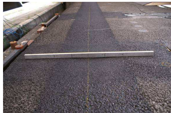
Rutting at N=80000. Left: +13 mm joint, right: -13mm joint.
