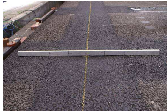
Rutting at N=70000. Left: +13 mm joint, right: -13mm joint.
