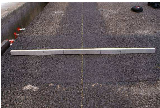
Rutting at N=20000. Left: +13 mm joint, right: -13mm joint.
