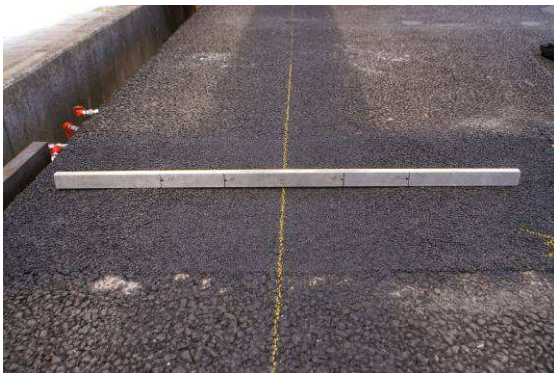
Rutting at N=10000. Left: +13 mm joint, right: -13mm joint.
