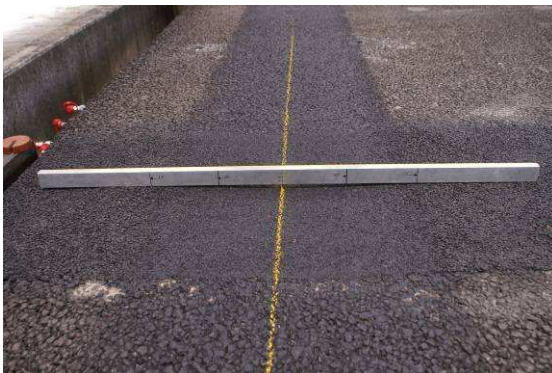
Rutting at N=70000. Left: +13 mm joint, right: -13mm joint.
