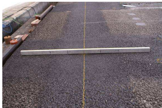
Rutting at N=50000. Left: +13 mm joint, right: -13mm joint.
