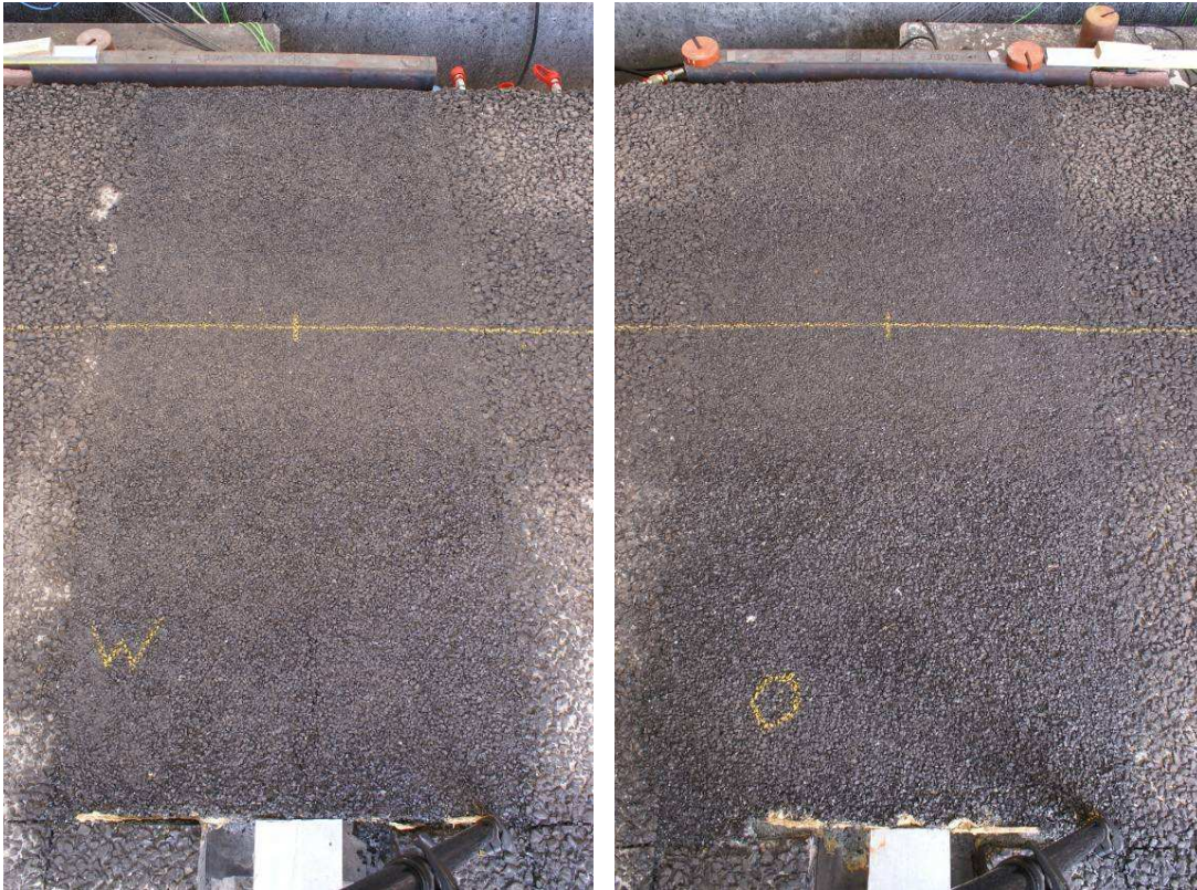
Top view at N=30000. Left: +13mm joint, right: -13mm joint.
