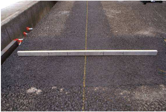
Rutting at N=30000. Left: +13 mm joint, right: -13mm joint.
