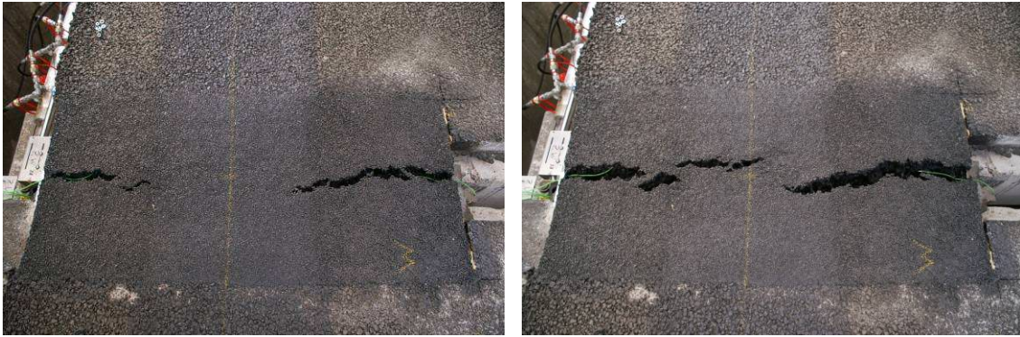
Left: t=2280 s, u= 63.5 mm, Right: t= 2880 s, u= 91.28 mm
