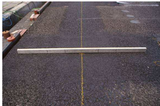
Rutting at N=40000. Left: +13 mm joint, right: -13mm joint.
