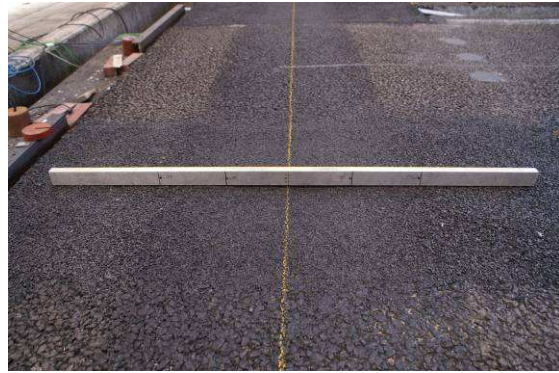
Rutting at N=30000. Left: +13 mm joint, right: -13mm joint.
