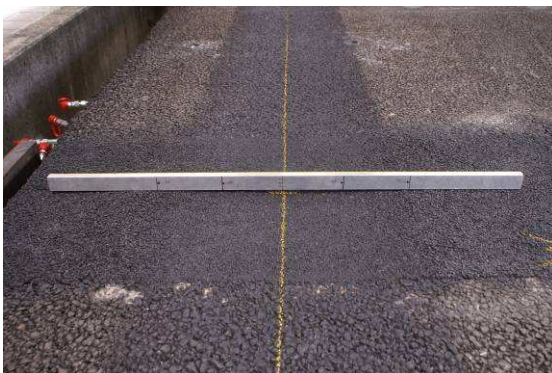
Rutting at N=50000. Left: +13 mm joint, right: -13mm joint.
