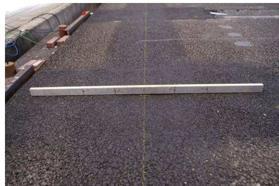
Rutting at N=20000. Left: +13 mm joint, right: -13mm joint.
